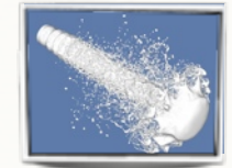
Atomization of a pulsed liquid jet.
