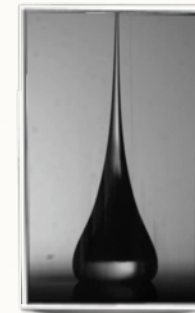
droplet impacting a superhydrophobic surface
